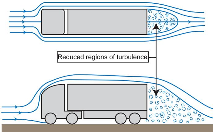
Substantial improvements in airflow around the vehicle can be achieved by relatively small modifications such as a modest curving to the front and side edges of the cab.
