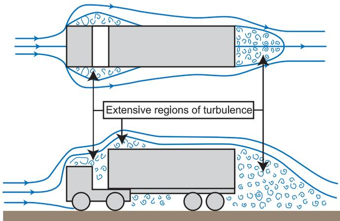
Figure 2 Typical Airflow Pattern around an Aerodynamically Effective Truck
